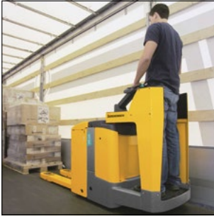
Protected operator workplace
